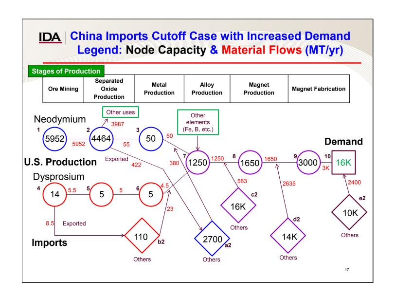
The next scenario modeled is one in which all imports from China are cut off and U.S. demand is increased (by 6.7 percent) to 16,000 MT of magnets. As with the previous case, the supply chain responds to try to meet U.S. demand for magnets under those conditions. Magnet shortfalls must be made up by mitigation measures.
