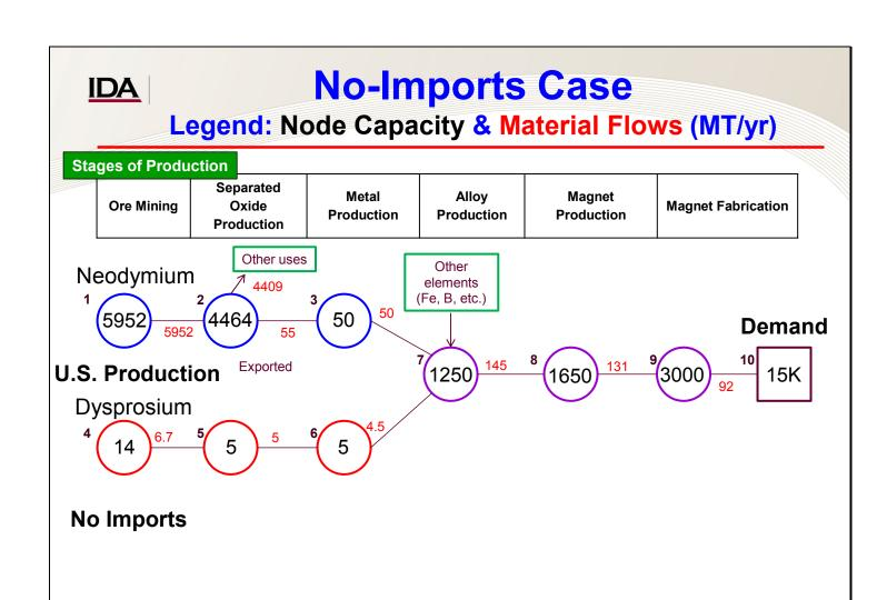
The next scenario modeled is one in which all imports are cut off completely (demand is reset to the previous figure of 15,000 MT of magnets). This case is something of an artificial case, but it shows how the method can address a broad range of possible supply and demand combinations. As with the previous cases, the supply chain responds to try to meet U.S. demand for magnets under those conditions.
