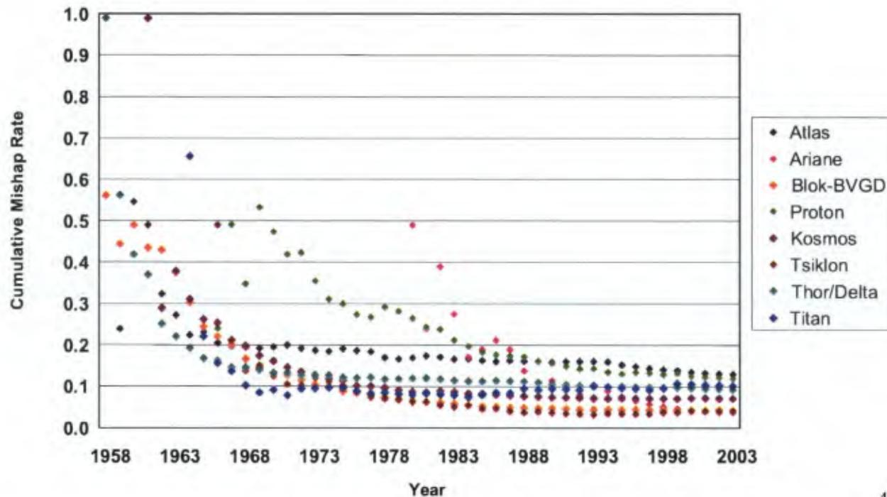
Further analysis of launch statistics revealed that the learning curve also appears to apply to separate launch vehicle families, indicating that launch vehicle operators also follow a learning curve as they gain experience with the vehicle.
