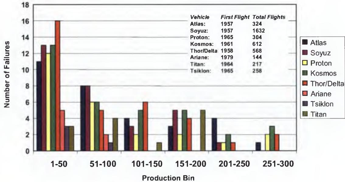
To understand the learning curve within families, STPI sorted launch failures from vehicle families according to total launches since the beginning of the vehicle program. While the failure statistics do not decrease monotonically with launch number, the overall trend of decreasing failure rates with launch number is apparent.
