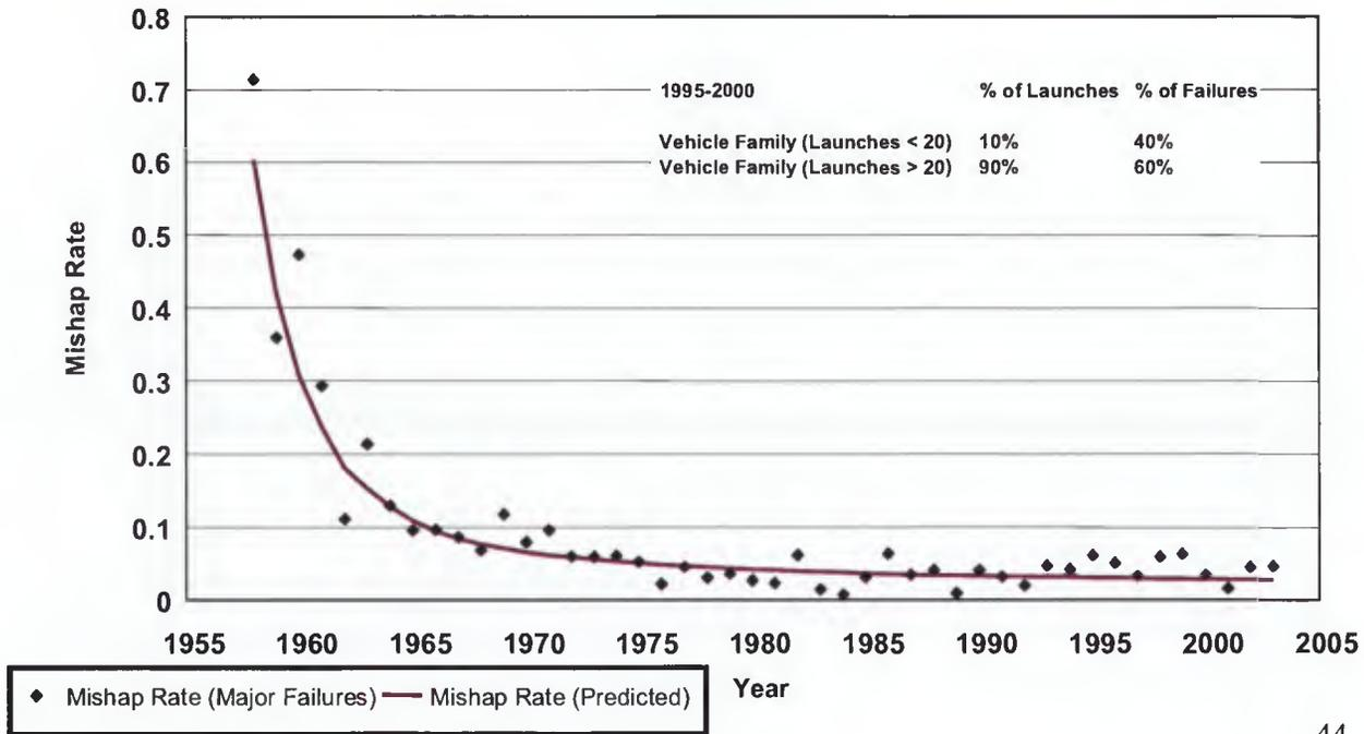
The historical launch vehicle mishap rate closely follows a standard learning curve: the mishap rate has fallen steadily over time from over 50% failures in the late 1950s to around 5% starting in the 1980s. The mishap rate has not noticeably decreased since then.
