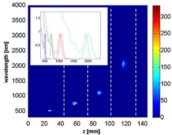
Absorption and emission spectra for each color segment are shown in the inset.
