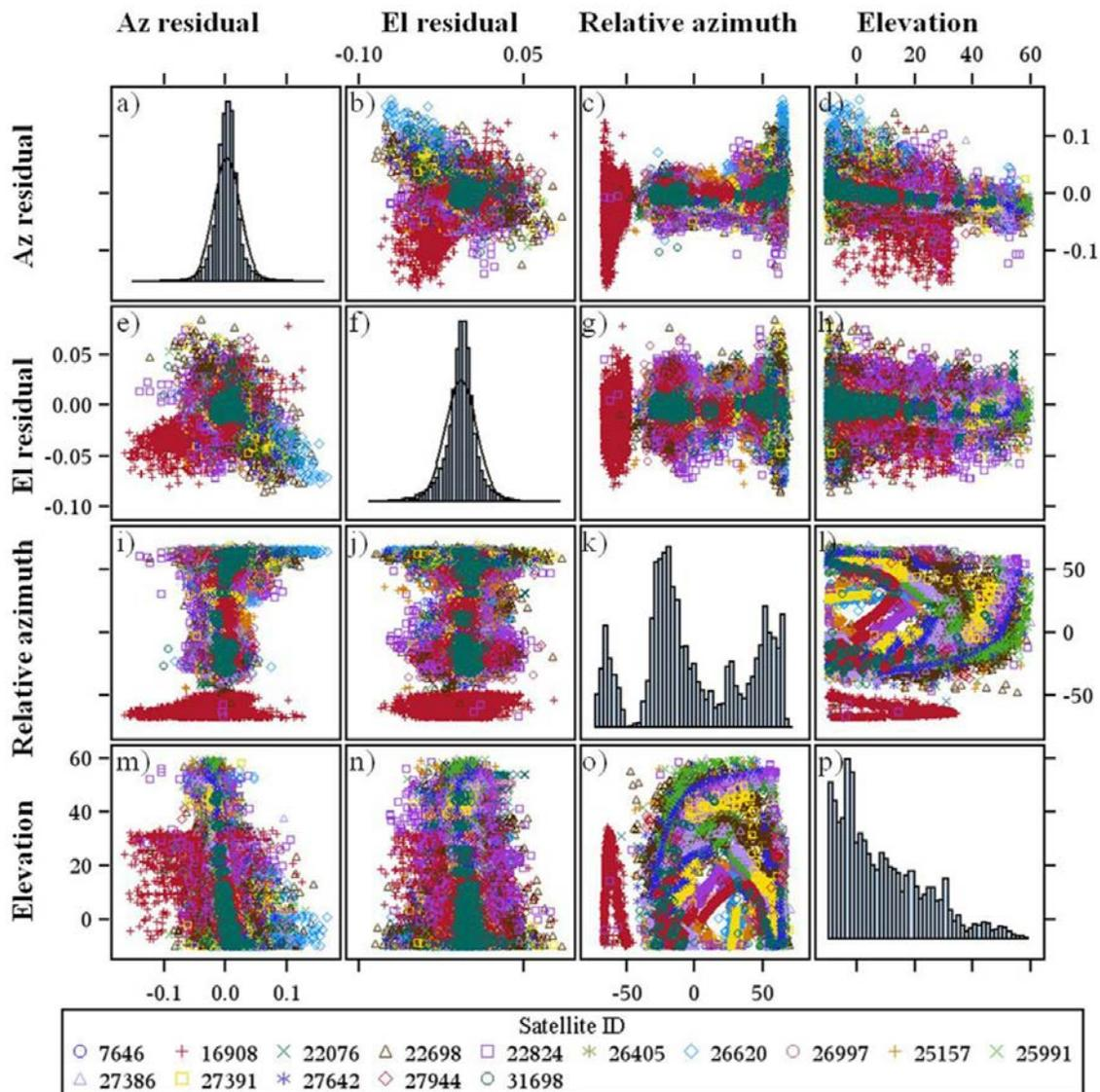
Figure 2. Summary of Cobra Data Calibration Satellite Observations Broken Down by Satellite ID.
