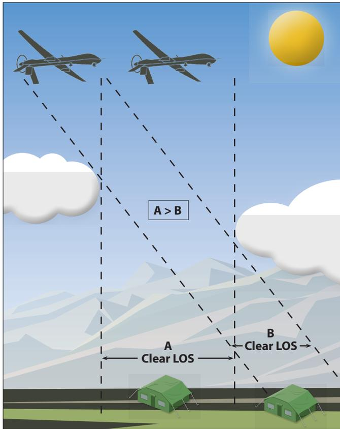
viewing a target off nadir, since the light path from target to sensor would pass through a greater amount of the cloud layer and thus have a higher probability of hitting a cloud. (See illustration.)
