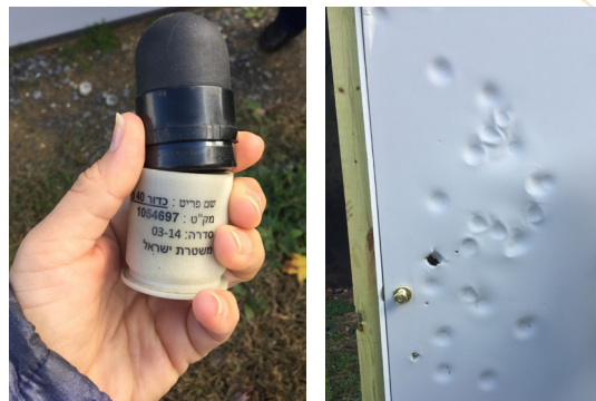
Source: Combined Tactical Systems (CTS). A steel slab exterior door with polyurethane core was the target in a demonstration of damage caused by 40-mm rubber rounds delivered by single- and multi-launchers with 5-inch cylinders. For details, see IDA YouTube .
