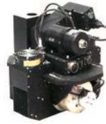
Argon Enhanced Airborne Multispectral Scanner (0.6 m r IFOV)
