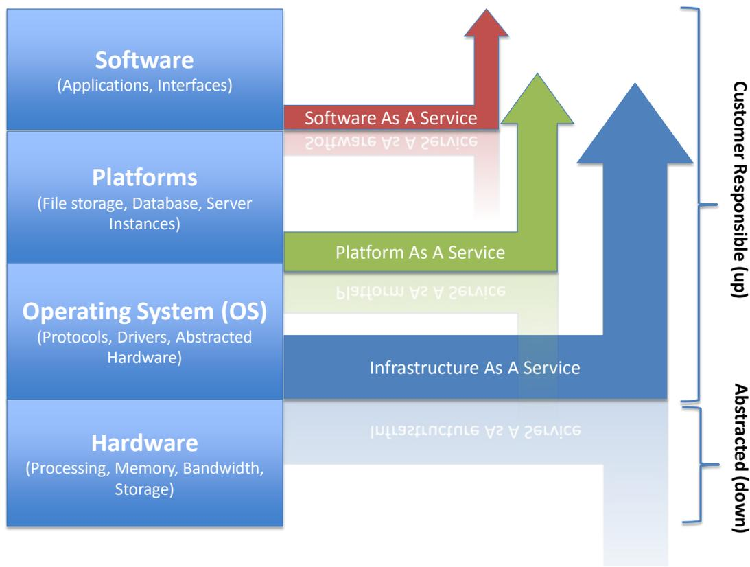
**Figure 10. XaaS and Abstraction of the Computing Stack**
