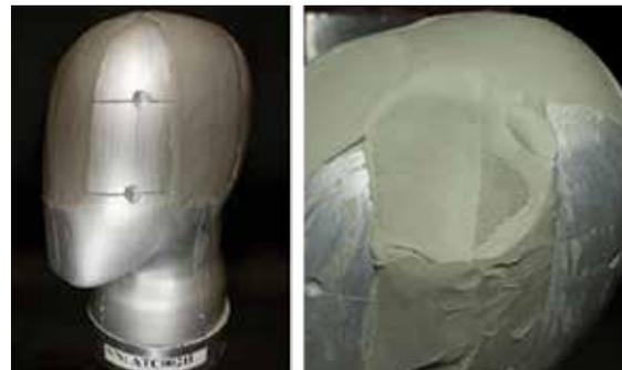
Figure 4. Clay Helmet Head Form Before the Shot (left) and After the Shot (right) Illustrating the Helmet Deformation into the Clay Channel
