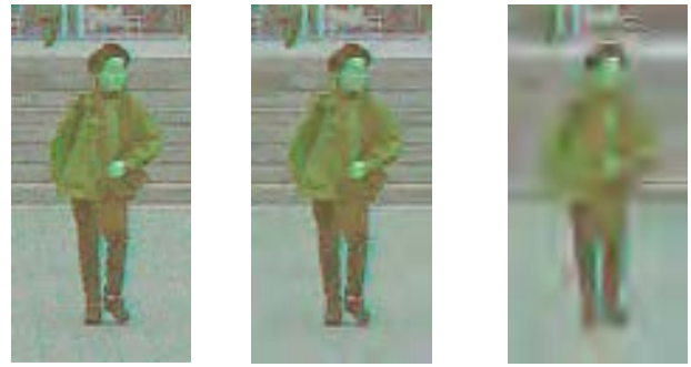
Fig. 5. Test image, at original scale: uncompressed (left), compressed at 16:1 (middle), and compressed at 64:1 (right).
