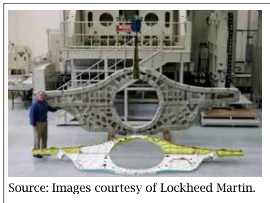
Figure 3. STOVL Bulkhead 496, Forged from Aluminum 7085
