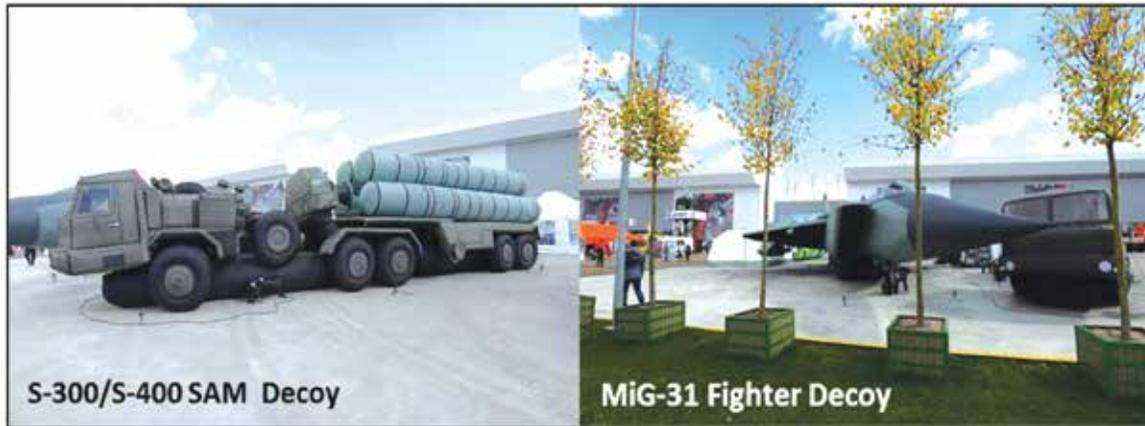
**Figure 7. Inflatable Decoys Displayed by Scientific Production Enterprise RUSBAL at ARMY-2016**
