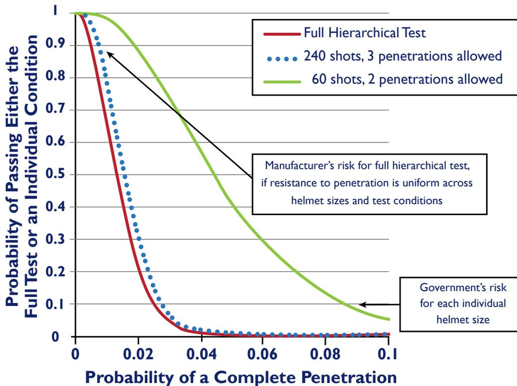
Figure 3. Operating Characteristic Curves for the DOT&E Aramid Helmet Protocol
