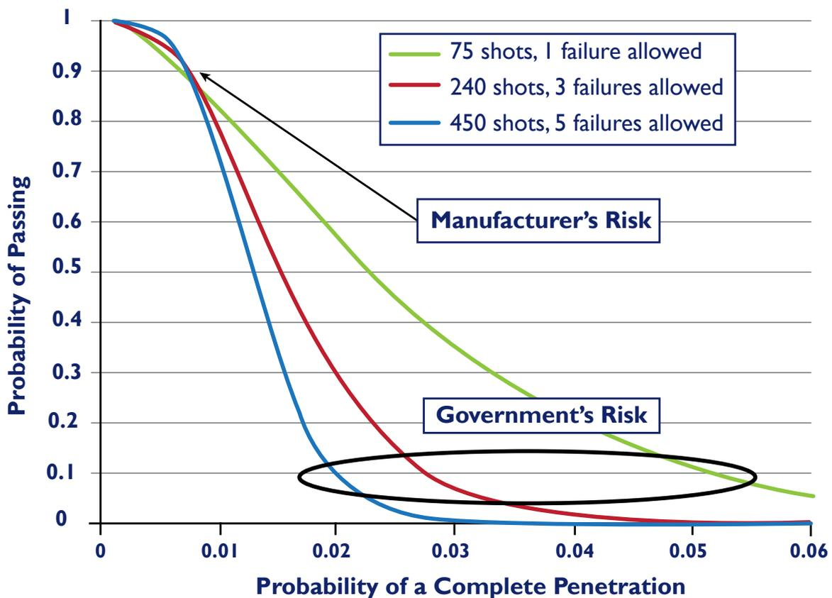
Figure 2. Operating Characteristic Curve for Test Sizes Ranging from 75 to 450 Shots
