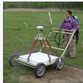
Collecting data with the Time-domain ElectroMagnetic Towed Array Detection System (TENTADS)
