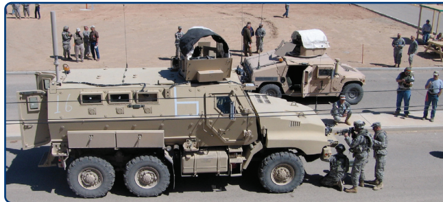
An MRAP vehicle (foreground), and a less protected HMMWV (behind) conduct operations in Yuma Proving Ground's "Little Baghdad" as OED and other test personnel observe the Initial Operational Test. Testing replicates environments and missions MRAPs might face in Iraq.
