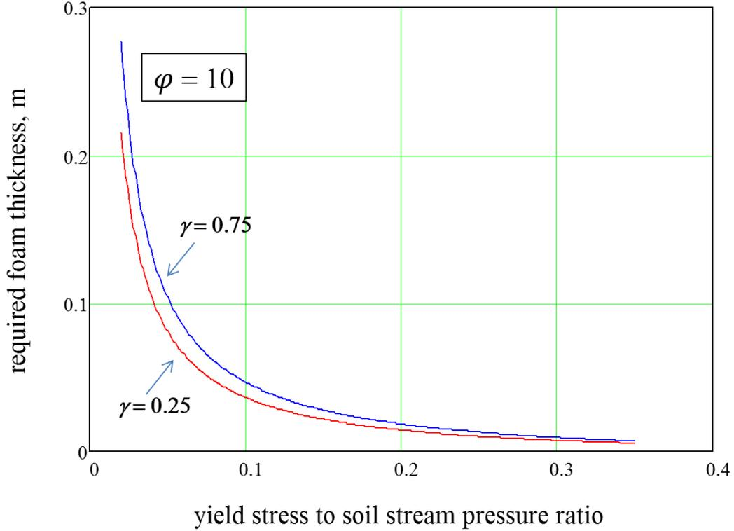
**Figure 11. Relationship between Required Foam Thickness and Yield Stress to Soil Stream Pressure Ratio**
