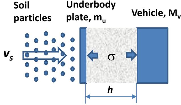
**Figure 7. Continuous Soil/Underbody Plate Impact Model with Resistive Force**
