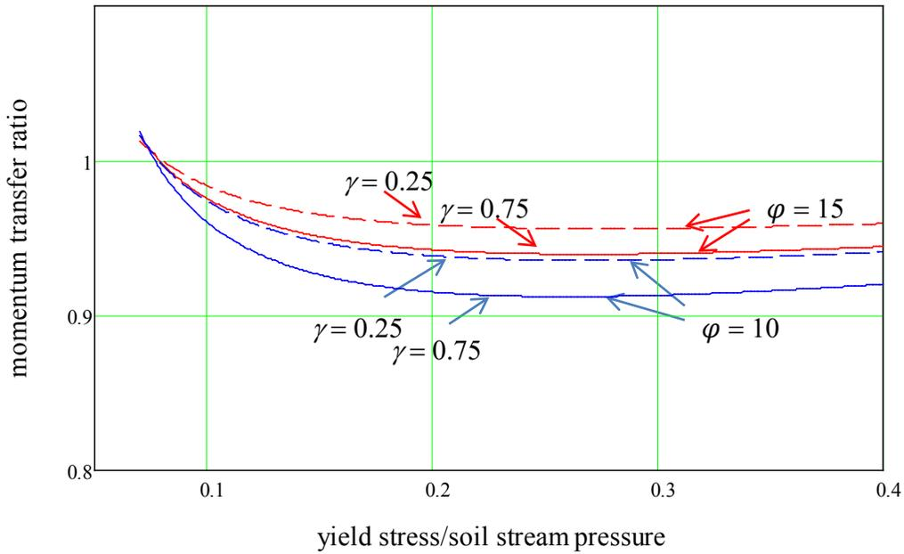
**Figure 12. Region of Optimum Values of Foam-Yield-Stress-to-Soil-Jet-Pressure Ratio**
