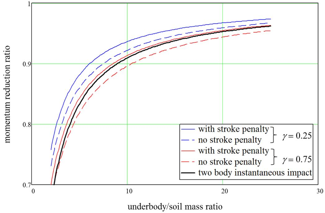
**Figure 13. Effect of Underbody-to-Soil-Mass Ratio on Momentum Transfer with Energy-Dissipation Stroke Penalty**
