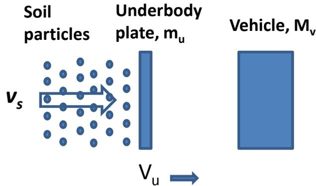
**Figure 5. Continuous Soil/Underbody Plate Impact Model**
