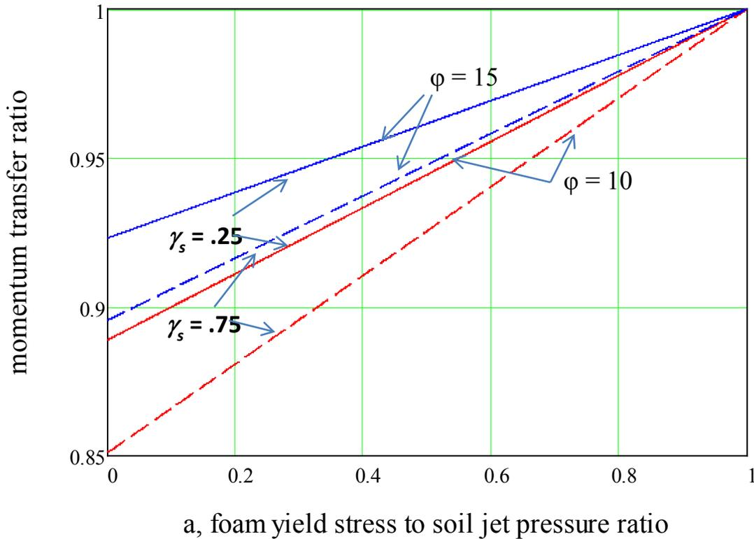
**Figure 9. Effect of Resistive Force on Momentum Transfer**
