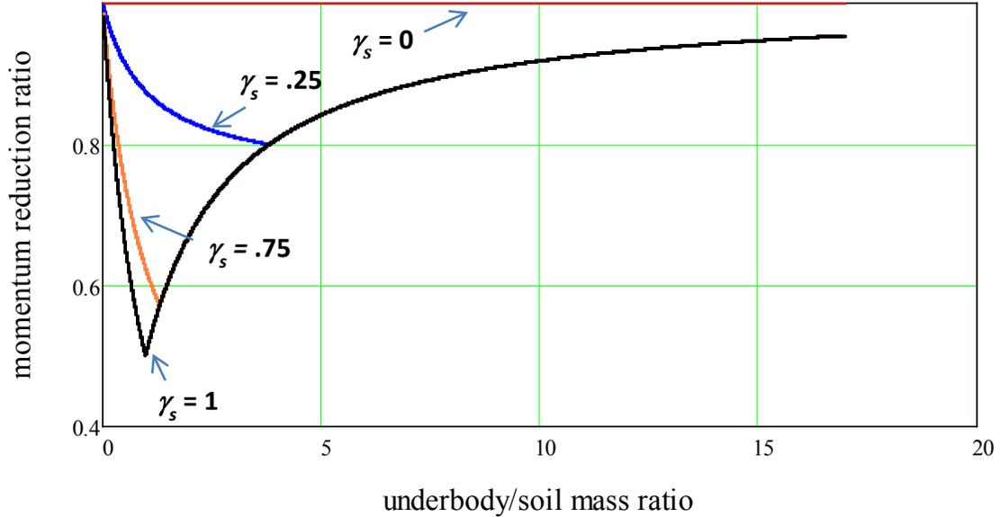
**Figure 4. Effect of Underbody/Soil Mass Ratio ( $\varphi$ ) on Vehicle Momentum-Transfer Ratio**
