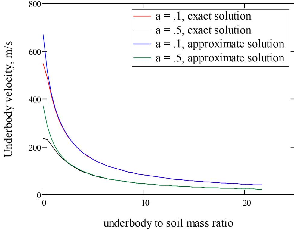
**Figure 8. Comparison of the Exact and Approximate Underbody Velocity Solutions**
