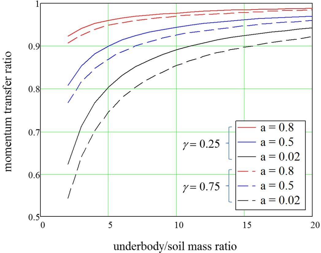
Figure 10. Effect of Underbody-to-Soil-Mass Ratio on Momentum Transfer
