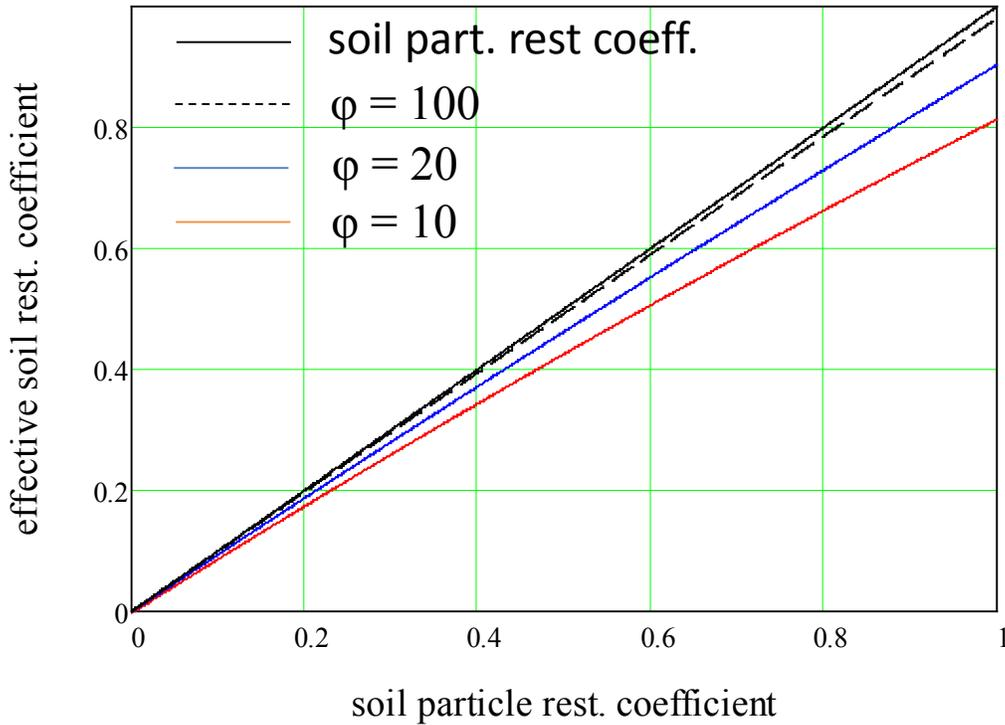
**Figure 6. Relationship between Soil Particle and Effective Restitution Coefficient**
