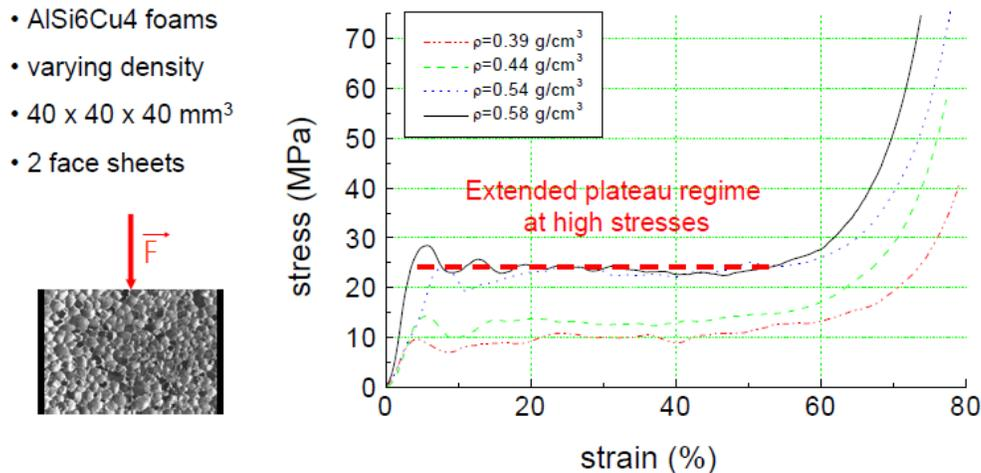
**Figure 1. Typical Stress vs. Strain Response of Aluminum Foams**
