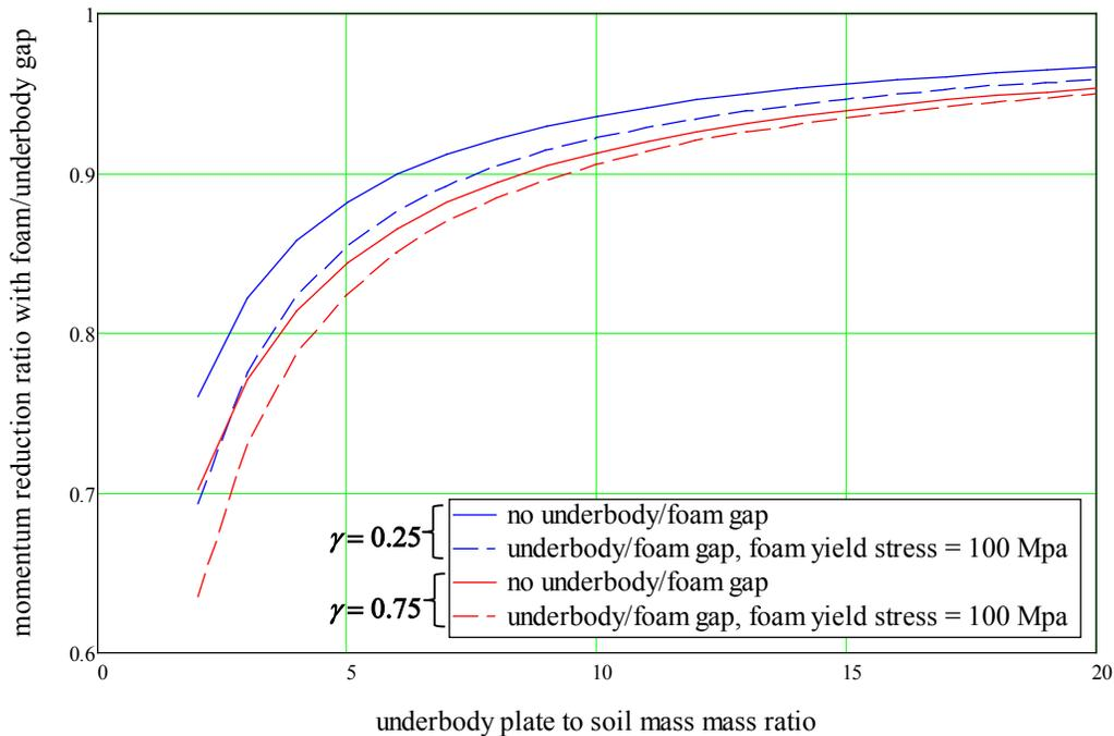
**Figure A-1. Comparison of the Momentum-Reduction Ratio for the Underbody/Foam “Gap vs. No Gap” Designs. No Gap design: underbody-to-soil-mass ratio,  $a = 0.3$ ; gap design:  $\sigma = 100$  Mpa.**
