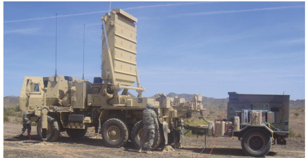
Soldiers Emplacing the AN/TPQ-53 (Q-53) Counterfire Radar
