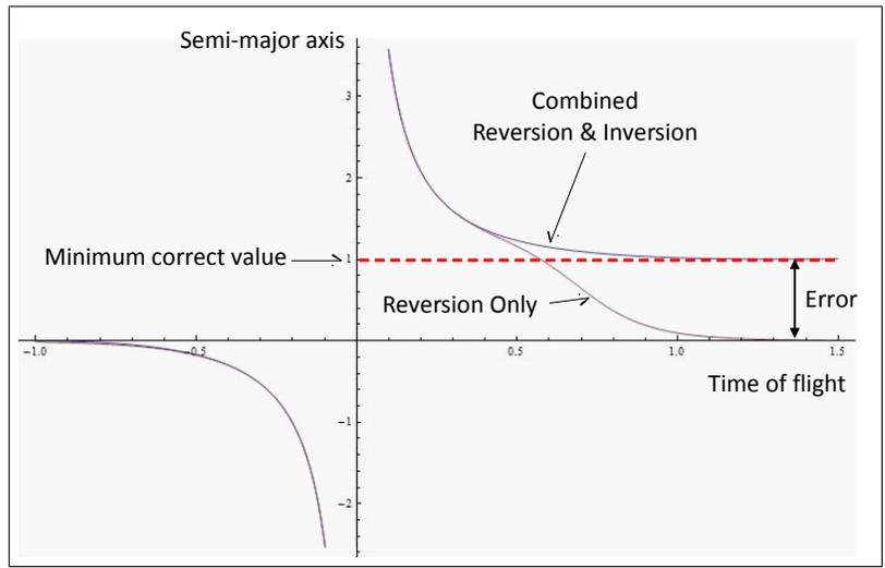
Figure 3: Series reversion combined with algebraic inversion
