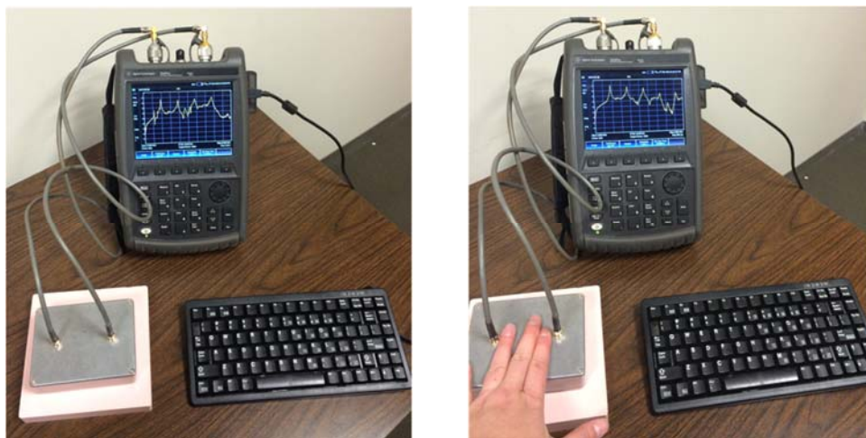
Figure 5: Taking a ring resonator measurement of RTV before and after applying pressure
