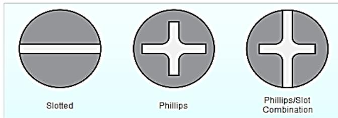
Screw is able to successfully function under multiple circumstances (different screw drivers)
