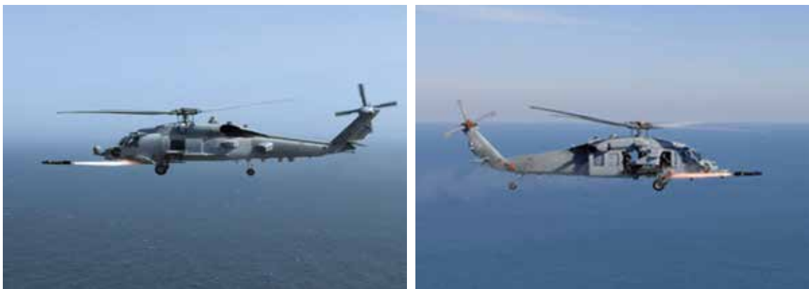
Figure 1. MH-60R (left) and MH-60S (right) Helicopters Employing AGM-114 Hellfire Missiles
