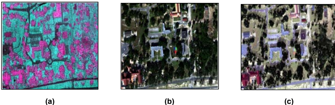
Figure 38. (a) Fusion of Depth-Intensity-Average Map from LiDAR; (b) with a Hyperspectral Image; (c) to Produce an HSI-LiDAR Fused Scene
