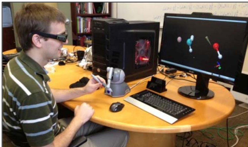
Figure 34. Interactive Ab Initio Molecular Dynamics with Haptic Force Feedback
