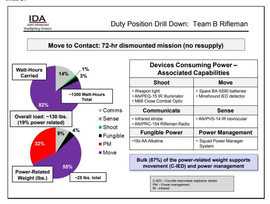
For this duty position, the power-related weight for C-IED dominates. Much of this move-related demand comes from the five spare BA-5590 batteries carried. These batteries weigh a total of 11.25 lbs. and they power the various C-IED devices carried by this Soldier and the rest of squad in this mission. For this particular mission, the Soldier also has to carry the one Squad Power Manager for the squad.
