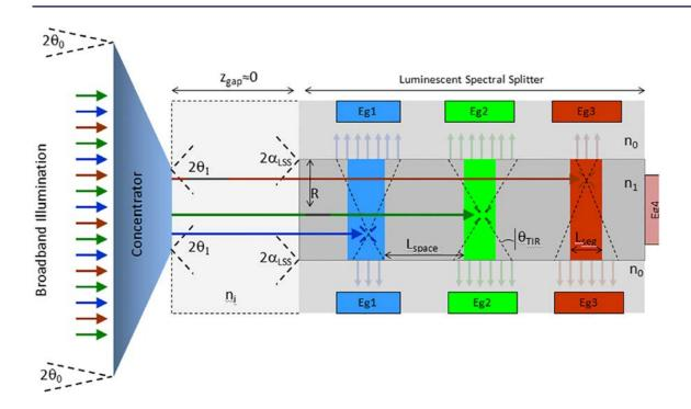
The gap between primary concentrator and the LSS is inflated so that angle definitions can be illustrated. The diagram is not to scale.
