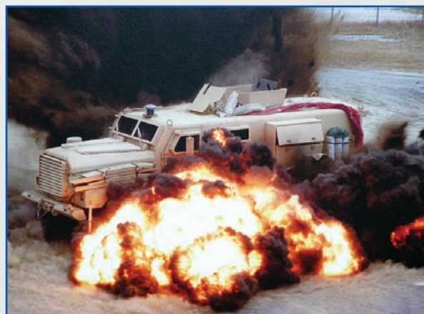
Figure 1: Testing of a Cougar Mine Resistant Ambush Vehicle.
