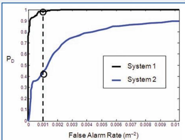
Figure 2: ROC curves for two GPR systems.
