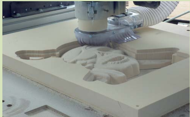
A COMPUTER NUMERICALLY CONTROLLED (CNC) ROUTING AND MILLING MACHINE STEERS A ROTATING BIT OVER A PIECE OF PLASTER TO CREATE THIS RELIEF DIRECTLY FROM AN ELECTRONIC BLUEPRINT. PICTURE TAKEN AT THE 2010 MAKERFAIRE
