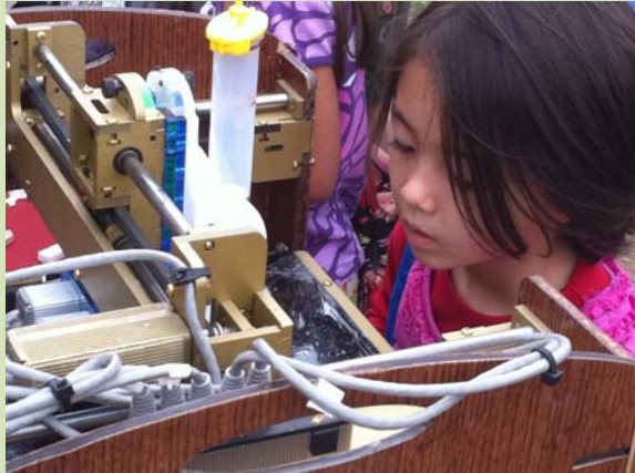
PERSONAL FABRICATION TECHNOLOGIES IN THE CLASSROOM APPEAL TO A BROAD RANGE OF STUDENT INTERESTS AND LEARNING STYLES. THIS 3 RD GRADER IS EXAMINING THE TOOLING MECHANISM OF A FAB@HOME 3D PRINTER AS IT CREATES A PLASTIC TOY. PHOTO TAKEN AT THE 2010 MAKERFAIRE
