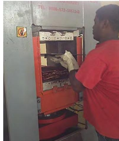
**Figure 5.11 Worker from African Bamboo using pressing machine on bamboo at pilot site**
